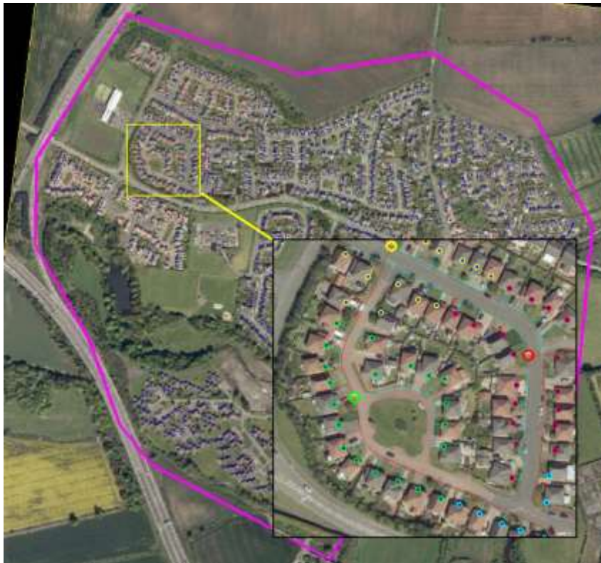
Picture: cost optimized DP and/or Cabinet area's, with cost optimized cable routes
